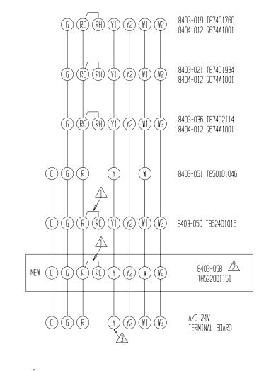
▲ FACTORY JUMPER ▲ THERMOSTAT DEFAULT SETTING IS FOR HEAT PUMP FOR HEAT/COOL GO TO SETUP FUNCTION 1, AND CHANGE SYSTEM TYPE TD "6", 2 HEAT/COOL. ▲ MAY BE DESIGNATED Y OR Y1 DEPENDING UPON SYSTEM
